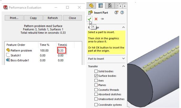
Instead of performing the Pattern of a Feature, the Pattern of a "Surface Body" is now used
