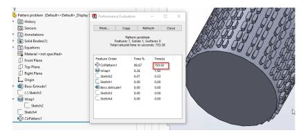
If you look at the Cirpattern1 feature's Options, the "Geometry Pattern" is not activated. With this option set, the time is reduced to 160 seconds. "Geometry Pattern" does not calculate each feature as an independent extrusion, but only the location itself. This setting alone provides an improvement of a factor of 4.5
