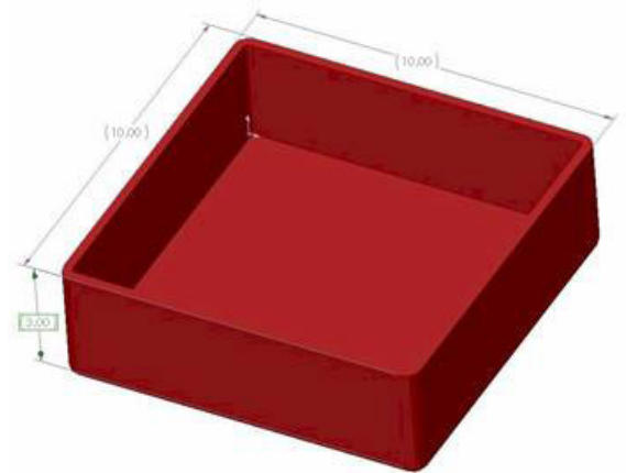
Size Limits for rapid injection molding is 20" x 20" x 3"
